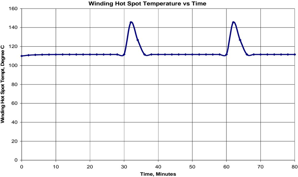
Figure 6: Calculated Winding Hot Spot Temperature due to GIC profile described above
