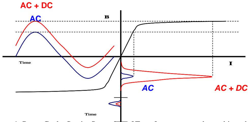
Figure 1: Part – Cycle, Semi – Saturation of Transformer cores when subjected to DC
