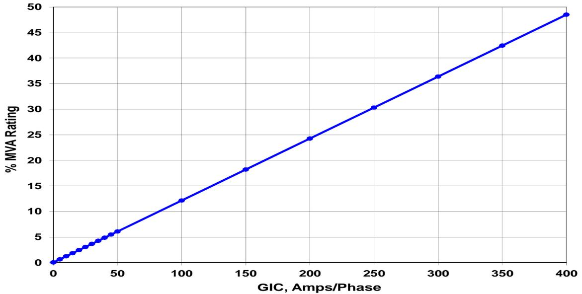
Figure 2: Calculated reactive power drawn by a large Transformer subjected to GIC
