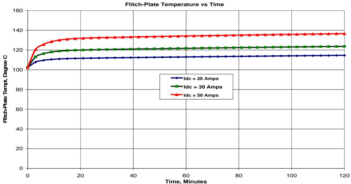
Figure 4: Calculated Flitch – Plate hot spot temperature for three values of DC
