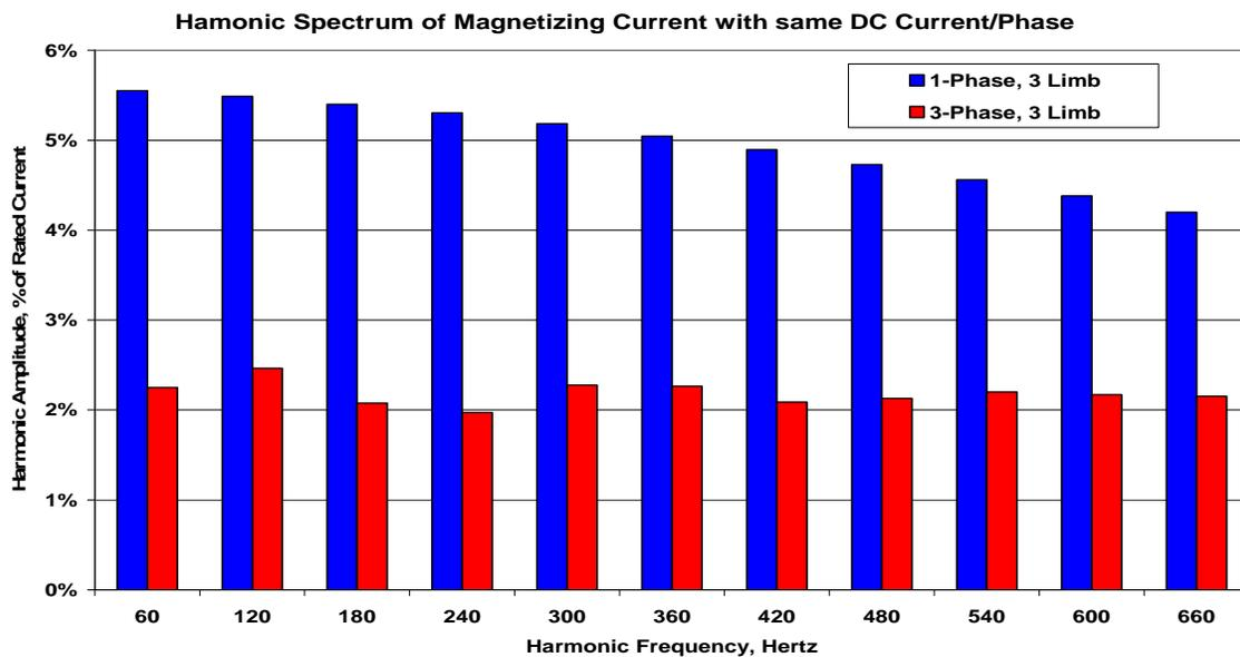
Figure 3: Harmonics of magnetizing current of transformers subjected to 30A/phase GIC
