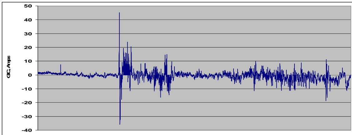
Figure 5: Measured GIC at a GSU transformer; during a 7 hours period
