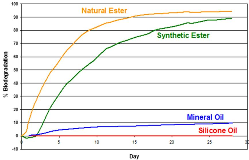
Fig. 1 : Biodegradability of various insulating fluids
