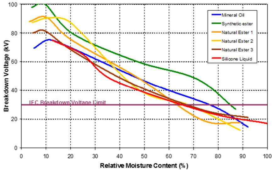
Fig. 2: Breakdown voltage related to relative humidity
